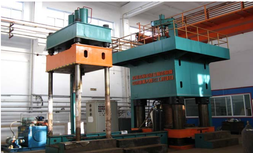
Figure 1.: 20MN servo control High temperature Triaxial pressure rock testing machine
